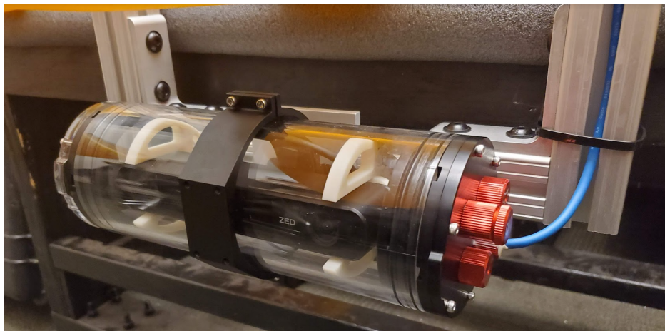
Figure 6: ZED 2i mounted within the BlueRobotics 3in Watertight Enclosure.
