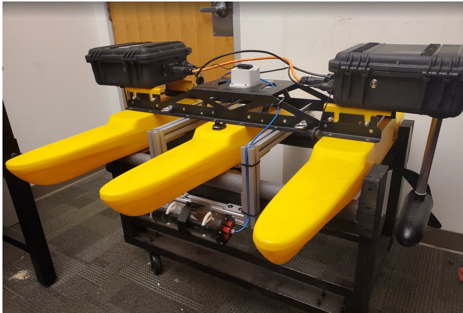
Figure 10: Final implementation of the ZED 2i mounted on the underside of the Kingfisher M100 inside the waterproof enclosure.
