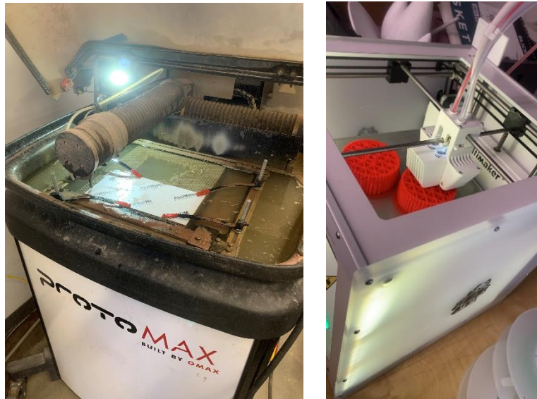
Figure 4226: Waterjet of Suspension Bar and 3D Printing of Drive Pulleys
