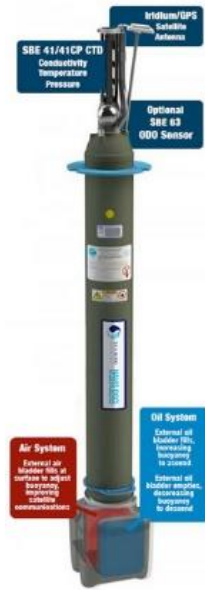
Figure 2. The Sea-Bird Scientific Navis Profiling Float, utilizing a mechanical displacement pump for its buoyancy engine and an external air bladder for better surface communications.
