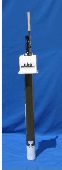
Figure 4. The NKE ARVOR I, a midrange “standard” float offered by NKE that collects CTD and pressure data and can operate at depths up to 2000 m.
