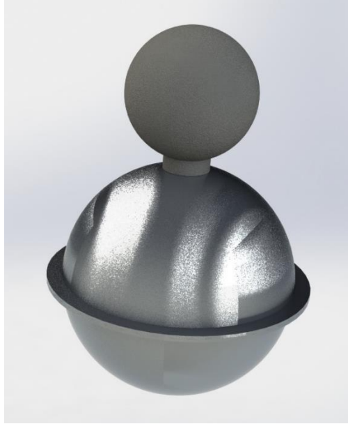
Figure 17. Concept of a flanged spherical design with an external oil sack serving a purpose similar to that of a hydraulic bellows.
