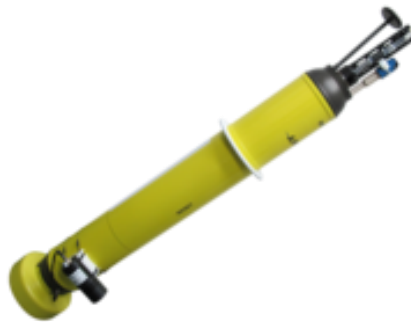
Figure 5. The Teledyne Marine APEX BioGeoChem float, a large and robust vehicle designed to support biogeochemical profiling for various research applications.
